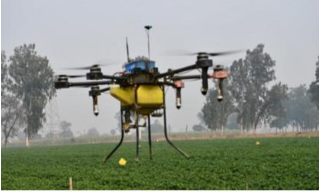
Drone based spray of chemicals
